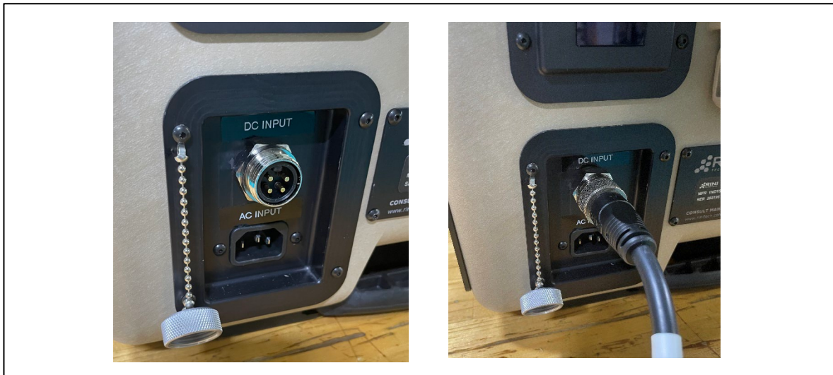
Figure 9: DC Power Connection
